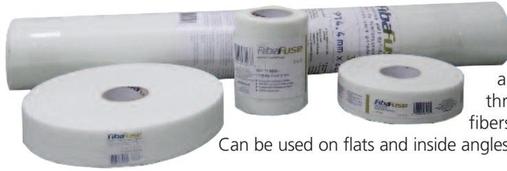
An innovative glass mat paperless drywall joint tape engineered with a porous, open fiber design that allows joint compound and other setting-type compounds to flow through and bond with the reinforced glass mat fibers, as well as the underlying work surface.
